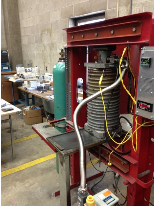
Figure 19. (a) Samples being heated in the furnace under vacuum followed by pressurizing with Ar.(b), (c) Pressure infiltration setup available at the Composite Center, University of Wisconsin-Milwaukee
