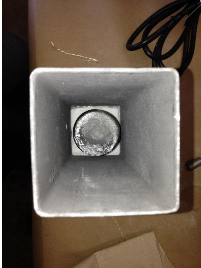
Figure 25. After placing the filter on top of the reinforcement, the metal is placed on top of the filter inside the mold.
