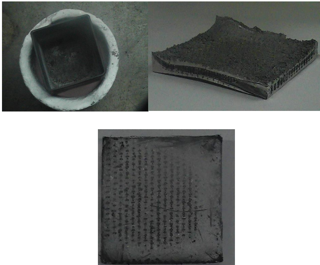
Figure 27. A typical MMC sample created after the PIP experiment.
